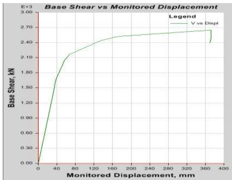
Fig 5. BASE Shear, Displacement
