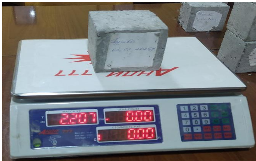
Figure 1. 28-day sample made from concrete mix with steel slag \phi 5 mm small aggregate
