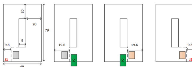
Figure 1: Four individual IPT turns, dimensions, and interconnecting points(mm)
