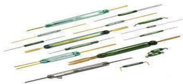
Fig.1. It is made up a pair of flattened ferromagnetic strips (reeds) which are hermetically sealed in a tiny glass tube.
